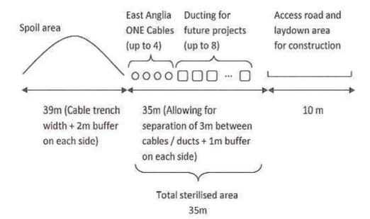
Diagram 2: Illustration of Potential Multiple phase construction
